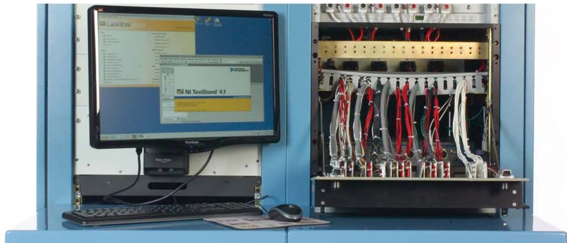
Front view of Tester showing Drop-Down Virginia Panel Interface for easy troubleshooting/repair/maintenance
