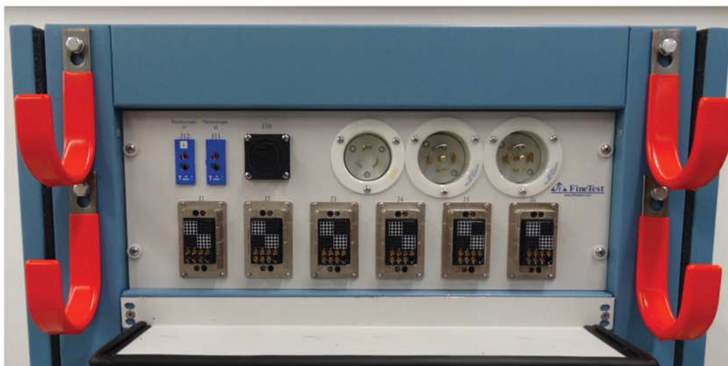
Rear System Interface Panel Close-Up showing Thermocouple Connections, AC Input Power Connections, 6 Unit Connections for Test Cables from Chamber to System, Cable Hooks for Test Cables
