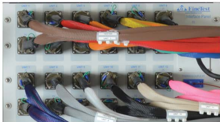
Rear System Interface Panel Close-Up showing 12 Unit Connections for Test Cables from Chamber to System
