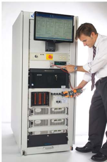
Cable Access in Front for Clip-On Meter
